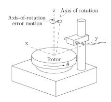
the remaining five degrees of freedom is referred to as an axis-of-rotation error motion or simply error motion. Depending on the error direction, one can distinguish two radial contributions, one axial and two tilt or wobble contributions. Furthermore, the error motion of stage can be separated into a synchronous and asynchronous component. The error motion of a stage is often incorrectly referred to as stage runout. A more elaborate explanation of these terms can be found here.
