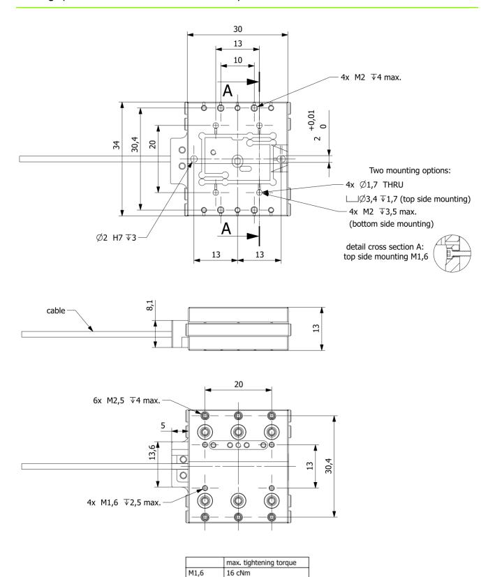
recommended flatness of mounting surfaces: 5 µm max.
